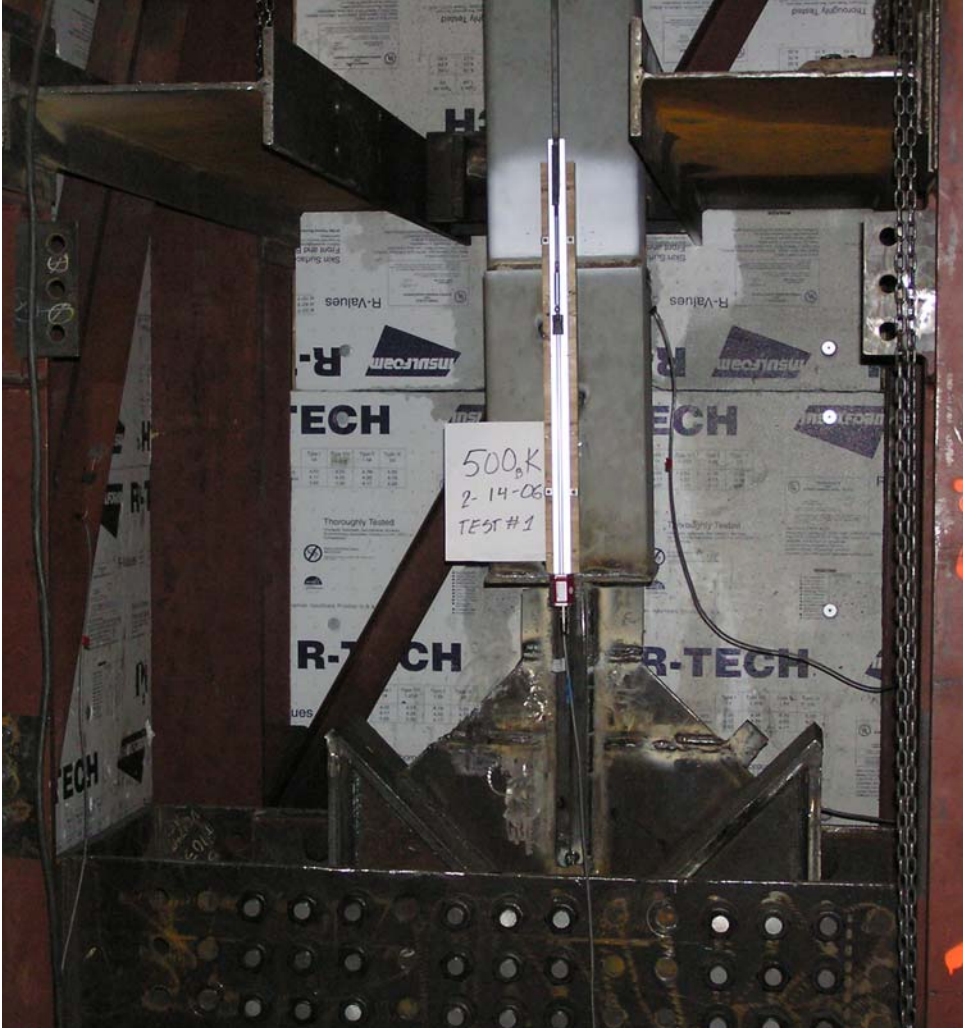
Figure 3 – Buckling Restrained Brace with LVDTs. The braces were installed 4” out of plumb to simulate frame drift. The LVDTs were welded to the brace.
